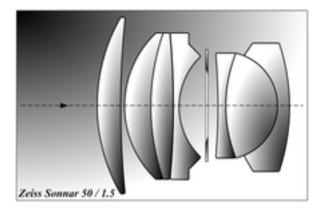
This diagram of the Zeiss Sonnar 50mm f1.5 has 7 optical elements in 3 groups. The Sonnar was first introduced in the 1930s and was known for its sharpness and light weight. Some variable focal length lenses have as many as 20 elements!
